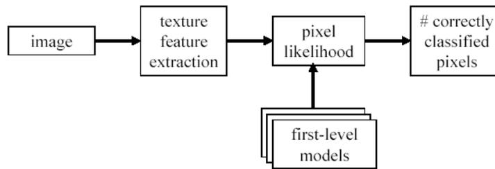
**Figure 3.** Classifying pixels using single-level motif models.
