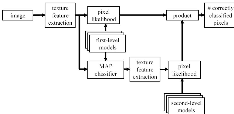
**Figure 4.** Classifying pixels using multiple-level motif models.
