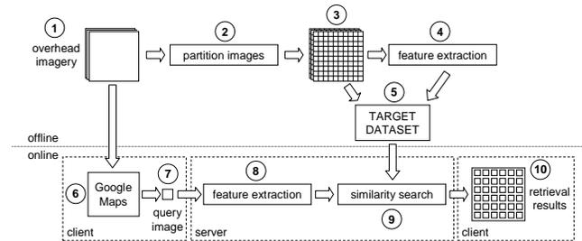
Figure 1: CBGIR system architecture.
